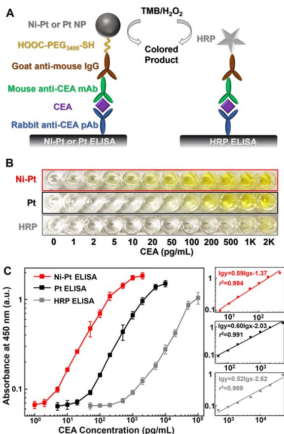
**Figure 4.** Detection of CEA with Ni–Pt NPs, Pt NPs, and HRP-based ELISAs. (A) Schematics of the three ELISAs of CEA. (B) Representative photographs taken from the ELISAs of CEA standards. (C) Corresponding calibration curves (left) along with linear range regions (right) of the detection results in (B). Error bars indicate standard deviations of eight independent measurements.
