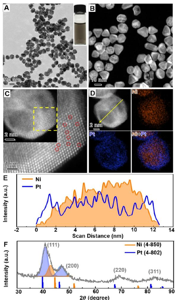
**Figure 1.** Structural and compositional analyses of Ni–Pt NPs. (A) TEM image, along with a photograph (inset) of the Ni–Pt NPs aqueous suspension. (B) HAADF-STEM image. (C) Atomic resolution HAADF-STEM image. Red circles highlight regions containing Ni atoms. (D) EDS mapping image and (E) EDS line-scan that were recorded from an individual NP shown in (D) along the direction indicated by the arrow. (F) XRD pattern.
