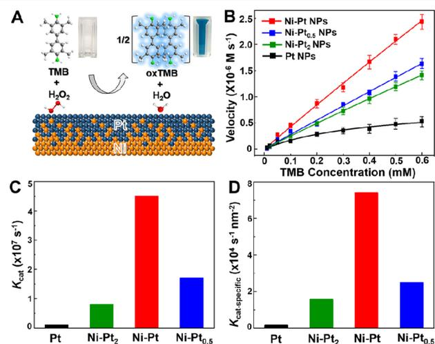
**Figure 2.** Peroxidase-like catalytic efficiencies of NPs with different Ni/Pt ratios. (A) Schematics showing the catalytic oxidation of TMB by H<sub>2</sub>O<sub>2</sub>. (B) Plots of initial reaction velocity for different NPs against TMB concentration. Error bars indicate standard deviations of three independent measurements. (C, D) Histograms comparing  $K_{\text{cat}}$  (C) and  $K_{\text{cat-specific}}$  (D) values of different NPs.
