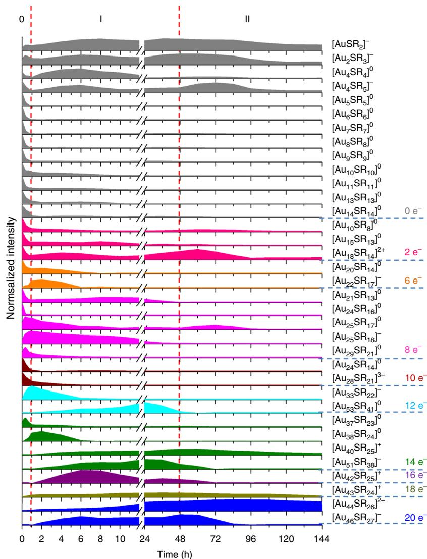
**Fig. 4** Time-dependent abundance of the as-identified Au(I)-SR complex/cluster species. The growth of  $[\text{Au}_{44}(\text{SR})_{26}]^{2-}$  can be divided into 3 stages: 0) kinetically dictated accumulation of  $\text{Au}_{25}$ , I)  $\text{Au}_{25}$ -mediated size growth, and II) thermodynamically controlled size-focusing
